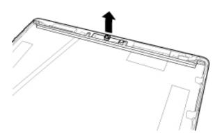
Figure 4-49 Removing the Camera
